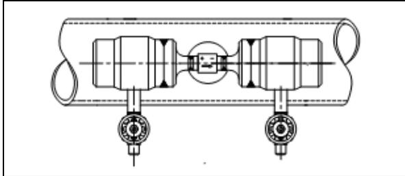
fig. 11: IBRD installed in a horizontal pipe
