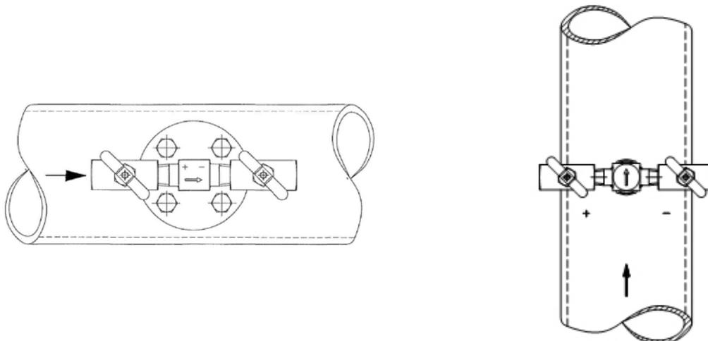
fig. 1+2: Arrangement of pressure tapping in horizontal and vertical pipes
