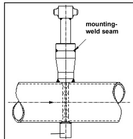
fig. 36 mounting weld seam IBFD-HTG
