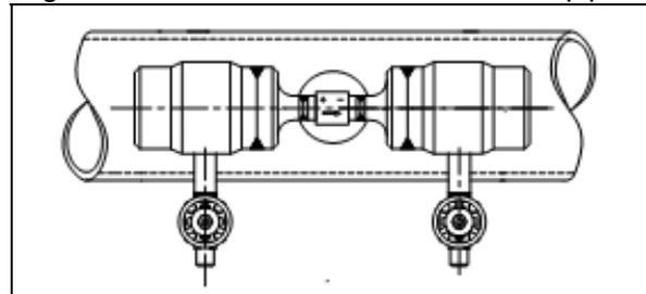
fig. 18: IBFD-26 HTG in a horizontal pipe
