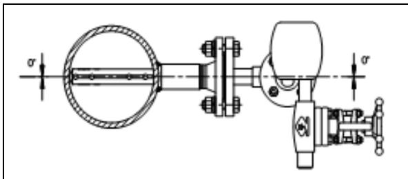
fig. 13: IBFD-25...-K1H-A81 in a horizontal pipe
