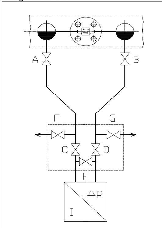
fig. 37 Sensor with condensate vessels K1
