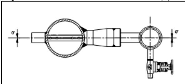
fig. 17: IBFD-26 HTG in a horizontal pipe
