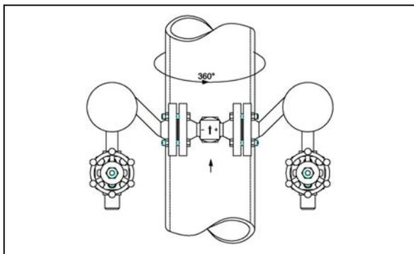
fig. 6: IBFD-25...-K1H-A81 in a vertical pipe
