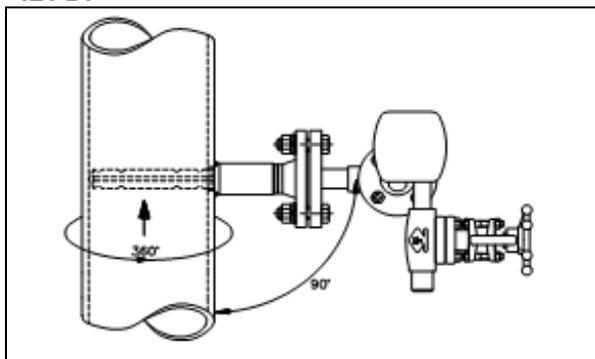
fig. 5: IBFD-25...-K1H-A81 in a vertical pipe
