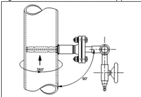
fig. 7: IBFD-25...-K7-A18 in a vertical pipe
