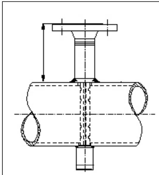
fig. 32: H-dimension for IBFD-HT-sensor
