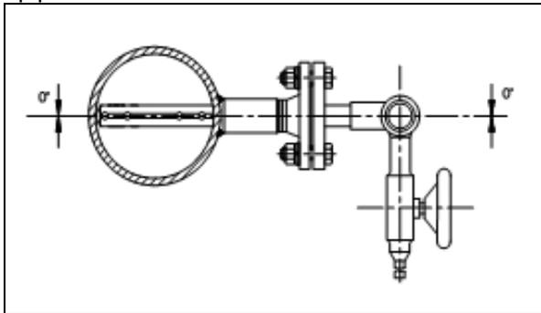
fig. 15: IBFD-25...-K7-A18 in a horizontal pipe
