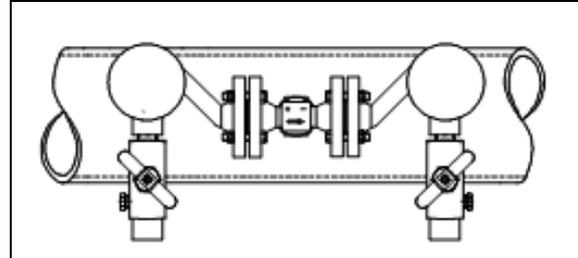
fig. 12: IBRD installed in a horizontal pipe
