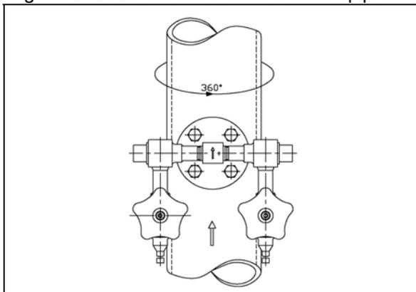
fig. 8: IBFD-25...-K7-A18 in a vertical pipe
