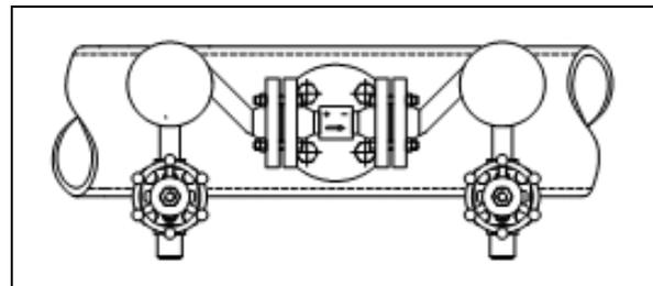
fig. 14: IBFD-25...-K1H-A81 in a horizontal pipe
