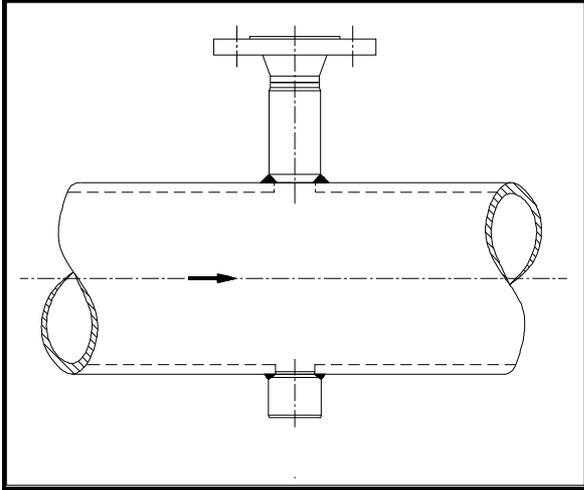
fig. 30 mounting parts sensor IBFD-21/26/36
