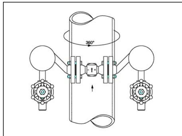
fig. 4: IBRD installed in a vertical pipe
