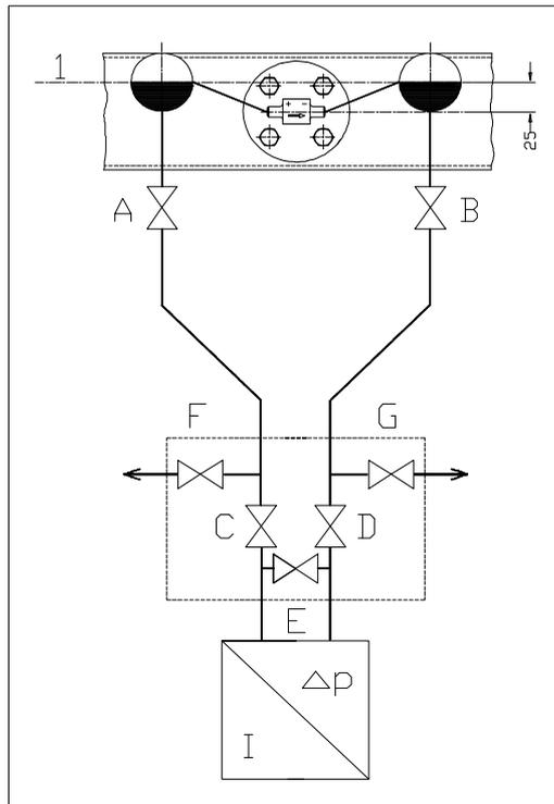
fig. 38 Sensor with condensate vessels K1
