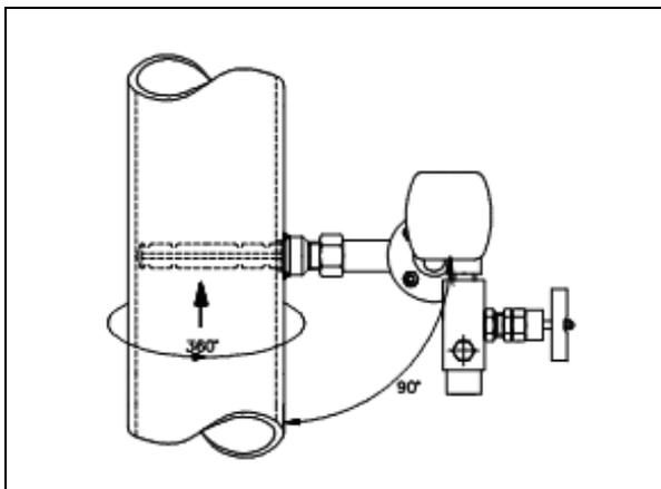
fig. 3: IBRD installed in a vertical pipe
