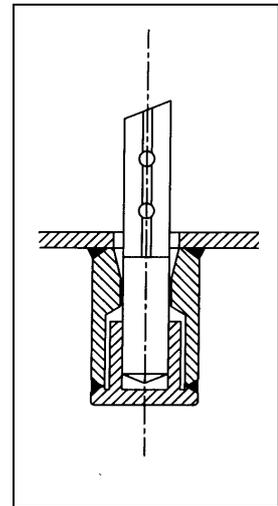
fig. 33: End support IBFD-HT, two-part welding construction
