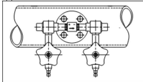
fig. 16: IBFD-25...-K7-A18 in a horizontal pipe
