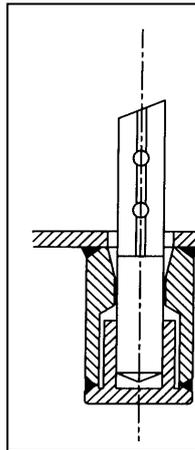
fig. 35 end support HTG-Sensor (two-part welding construction)
